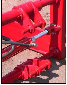
HOOK UP BRACKETS FOR LOADER ARE VERY UNIVERSAL. THE BRACKETS SLIDE ON A HEAVY KEYED TUBING FOR ANY WIDTH, TURN OVER FOR VERTICAL SPACING IF NECESSARY. THE BRACKETS ARE ALSO 2 PIECES SO SPACING CAN BE SET FOR LOADER ARM WIDTH.
