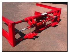
THIS PICTURE SHOWS THE REAR VIEW OF THE SQUEEZE, SHOWING THE CYLINDERS AND UNIVERSAL LOADER MOUNTING BRACKETS
