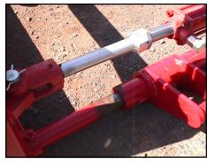
SQUEEZE CAN BE CHANGED FROM AN 8 TO 10 BALE (OR VICE VERSA) BY REMOVING OR ADD-ING CYLINDER EXTENSIONS, AND SHORTENING OR REPLACING SLIDE BARS.
