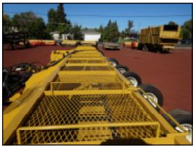
Large removable air screens provide excellent suction and allow easy access to the inside of machine for maintenance.
