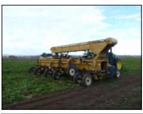
The optional elevator folds back for transportation and allows you to dump the material onto the ground.
