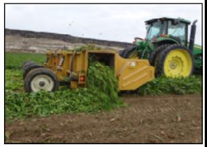
Conveyor drops the material to the passenger side of the machine. This allows you to windrow the tops of various crops for use in feeding applications.
