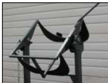
DUMP STAND ASSEMBLY. YOU CAN PLACE THE STAINLESS STEEL MATERIAL BASKET INTO THIS TO MAKE THE DUMPING OF THE COOKED MATERIAL QUICK AND EASY
