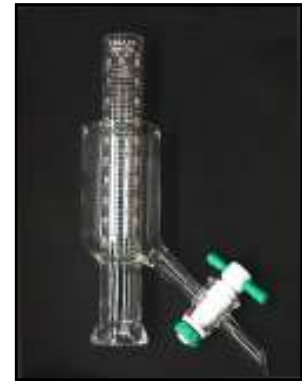
CLOSE UP VIEW OF GLASS BEAKER, SHOWS OIL/WATER LEVEL, OIL OVER FLOWS FROM SEPARATING TUBE INTO OUTER COLLECTION VESSEL THAT HAS A VALVE TO DISCHARGE OIL INTO A COLLECTION CONTAINER
