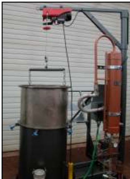
AN ELECTRIC HOIST IS PROVIDED TO LIFT THE STAINLESS MATERIAL BASKET OUT OF THE COOK POT ASSEMBLY AND INTO THE DUMP STAND ASSEMBLY.
