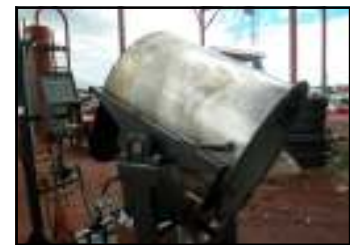
STAINLESS MATERIAL BASKET PLACED INTO THE DUMP STAND ASSEMBLY AND IN THE DUMP POSITION
