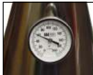
TEMPERATURE GAUGE ON THE TP RECEIVING CAN, FOR PROPER TEMPERATURE
