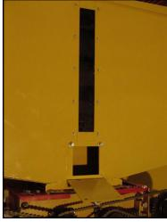
Grain level viewing window with a cleanout door. Adjustments to roller gap for different grains can be made from the clean out door.
