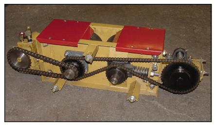
Hydraulic motor driven roller chain drive train for a positive roller drive. Spring loaded rollers with adjustable gap for different grains. Rollers are case hardened
