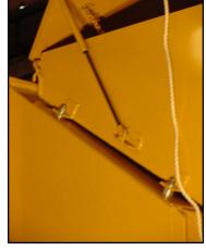
Crimp / Cracked grains can be diverted from chopper discharge chute to the outside chute for measuring or other use with the flipping of the lever above.
