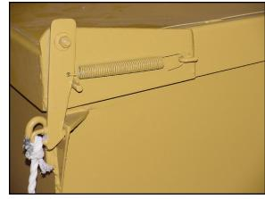
Rope is used from ground level to release latch and close gas spring assisted hopper lid.
