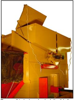
Rope pull to lock and unlock the lids for filling the hopper. Operated from ground level to avoid climbing up to open and close lids.
