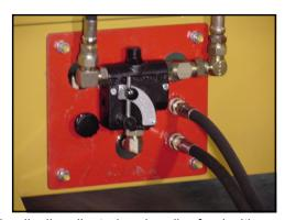
Hydraulically adjusted grain roller feed with a switching control knob which changes from the jack to the grain roller and back. Requiring only one set of hoses from the tractor to handle both functions.
